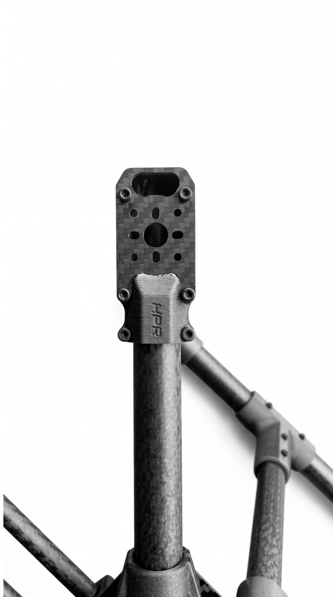
Motor mount detail – accepts 16, 19, 16×19, and 25 mm bolt circles.
