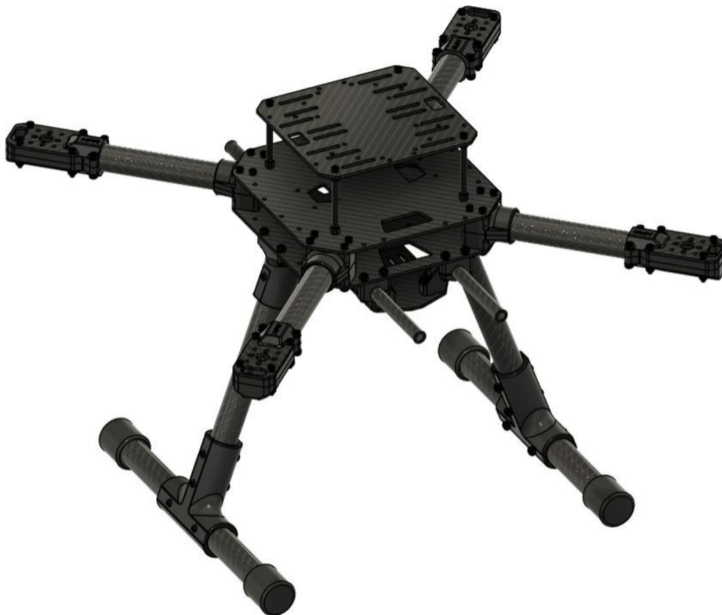
The completed Q500 airframe.
