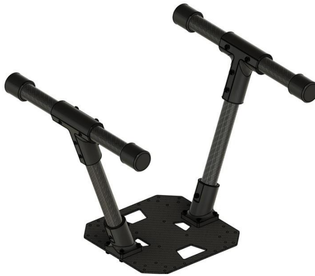
Both legs fitted, frame still upside down.
